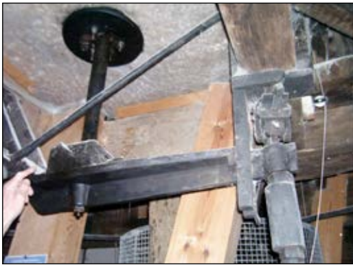
The screw controlled cantilever system that adjusts the gap setting by raising or lowering the bottom fixed stone.
