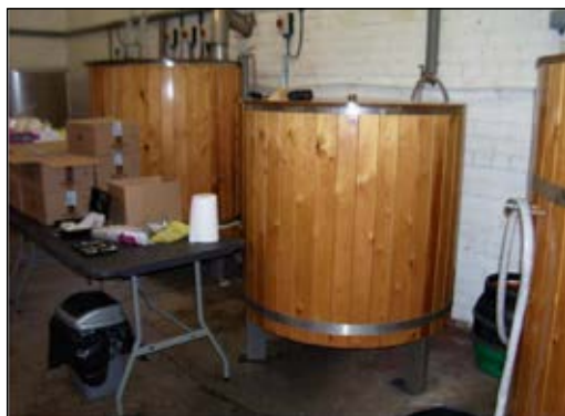
The 6BBL PBC kit: Left to right – Copper, mash tun and edge of HLT
